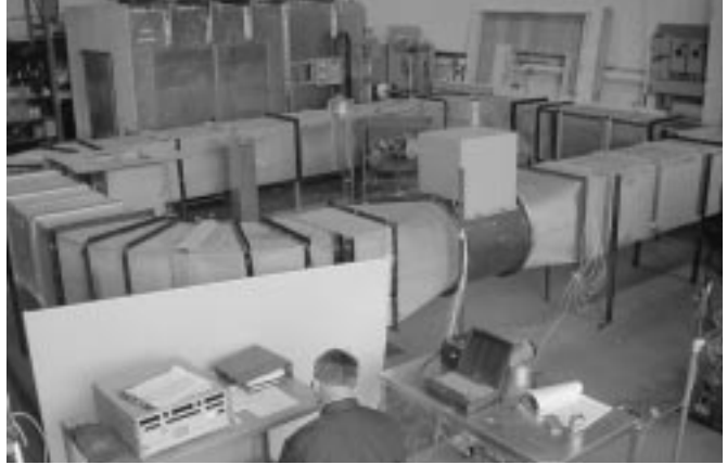
Photo of recent test on an inline smoke fan
