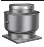
Model CUE is a direct drive exhaust fan specifically designed for roof or sidewall mounted applications discharging the air directly upward, away from the roof or wall surface. The fans feature a one piece windband continuously welded to curb cap and double studded isolators for true vibration isolation.
