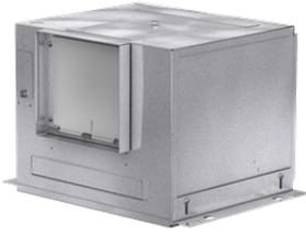
Model CSP inline fans are high performance fans designed for exhaust, supply or return air applications where low sound level are required. Units feature an insulated, galvanized steel housing with a forward-curved wheel.
