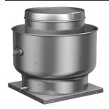
The CUBE is an aluminum exhaust fan specifically designed for roof or sidewall mounted applications where contaminated or grease laden exhaust air can be discharged directly upward, away from the roof or wall surface. The fans feature a one piece windband continuously welded to curb cap and double studded isolators for true vibration isolation.
