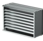
Brick vents provide a permanent means of ventilation for crawl spaces, hung ceilings, incinerator rooms, chimney flues, foundations, pipe spaces and corridors. Extruded construction provides a quality finished appearance. A high water stop at the rear and deep overlapping blades with storm stops provide maximum resistance to rain and weather.
