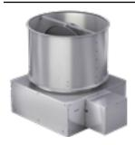
The RBUMO is an upblast axial exhaust fan designed to discharge air and contaminants up and away from the roof surface for most commercial and many industrial applications. This belt-driven fan features a welded steel propeller designed to run at lower RPMs, generating low sound levels, making the RBUMO the ideal solution for sound critical installations. The motor is located outside of the airstream to allow for high temperature air to be exhausted as well as roof access to the motor.
