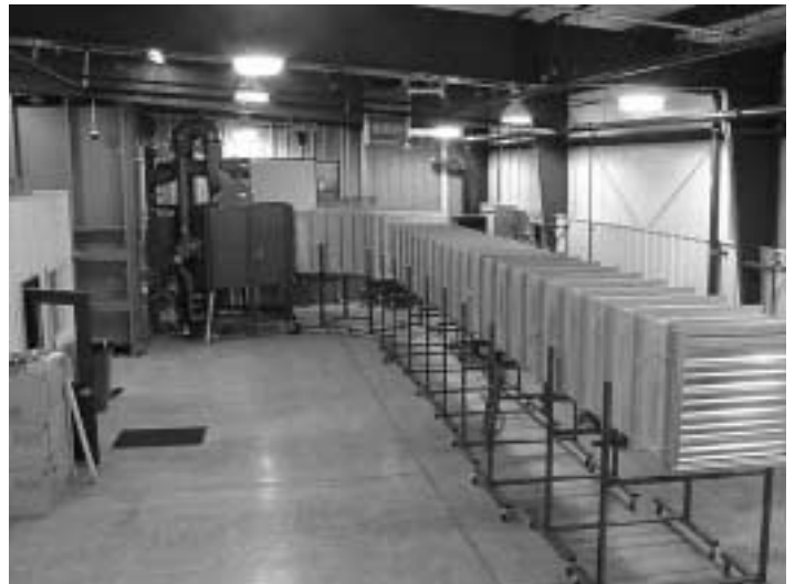
Pictured above is Greenheck's UL-certified on-site testing lab, where the manufacturer's smoke and fire dampers are tested with heated air to simulate fire emergency conditions. This testing procedure is required by new UL Standards.
