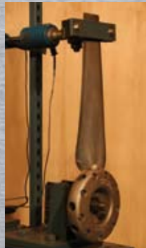
Fatigue Blade Cycle Test
