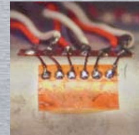
Strain gage on axial fan aluminum hub.
