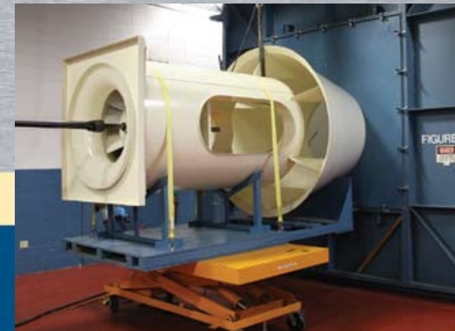
A laboratory exhaust fan undergoes air performance analysis.
