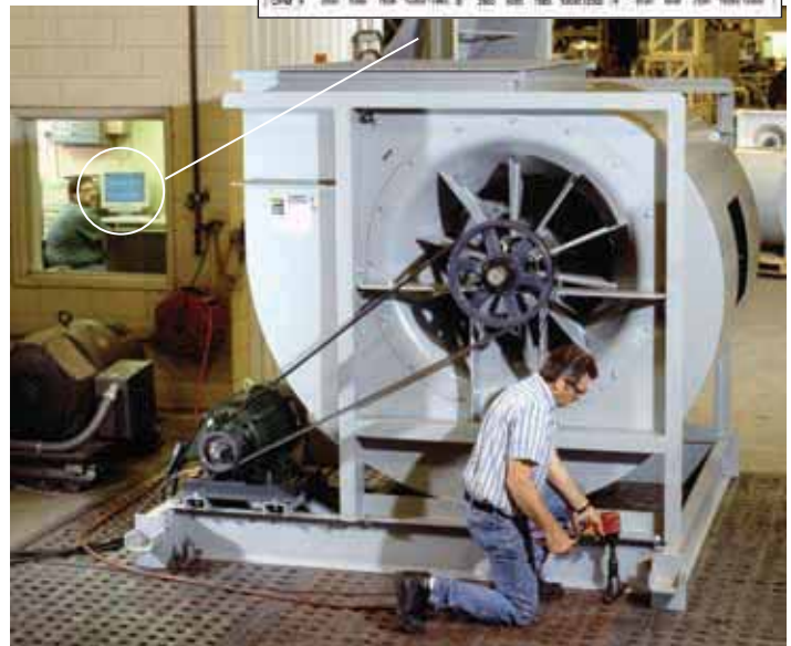
Assembled Fan Package on Vibration Test Stand
