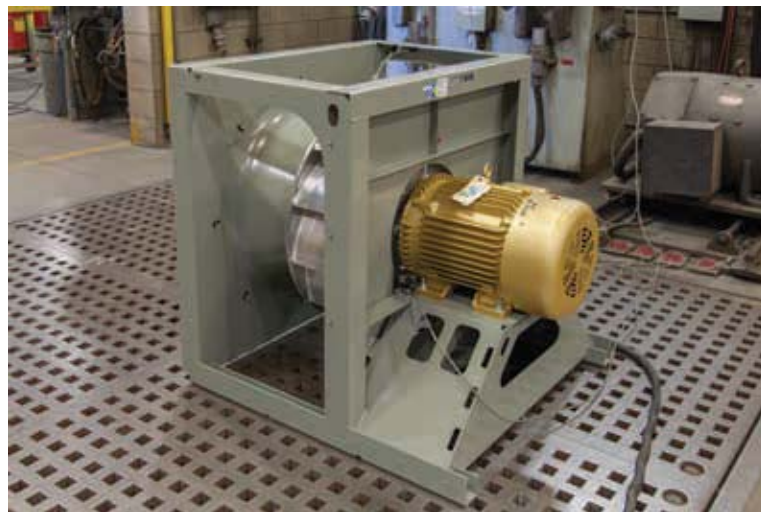
APH Arr. 4, Horizontal, shown being vibration tested
