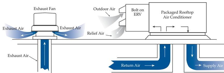
exhaust air code required is roughly half of the outdoor air volume. This means compared to the bolt-on unit, the stand alone ERV can recover energy from twice as much air leaving the building. The net impact is nearly double the effectiveness for the stand alone system.
