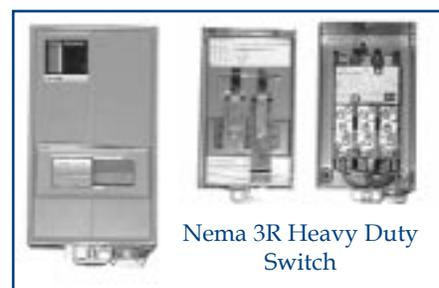
**NEMA 3R:** Enclosure constructed for either indoor or outdoor use to provide a degree of protection to personnel against incidental contact with the enclosed equipment: to provide a degree of protection against falling dirt, rain, sleet, snow, and windblown dust. The enclosed equipment will be undamaged by the external formation of ice on the enclosure. The NEMA 3R enclosure meets the rod entry, rain, external icing, outdoor corrosion protection and gasket design tests.
