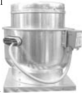
Greenheck's CUBE-180 upblast roof fan shown with a NEMA 3R disconnect, exterior mounted and factory wired to the motor with non-metallic liquid tight conduit.
