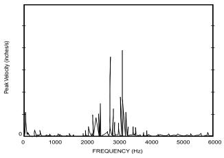
Example of vibration spectrum showing "Bearing Fluting"
